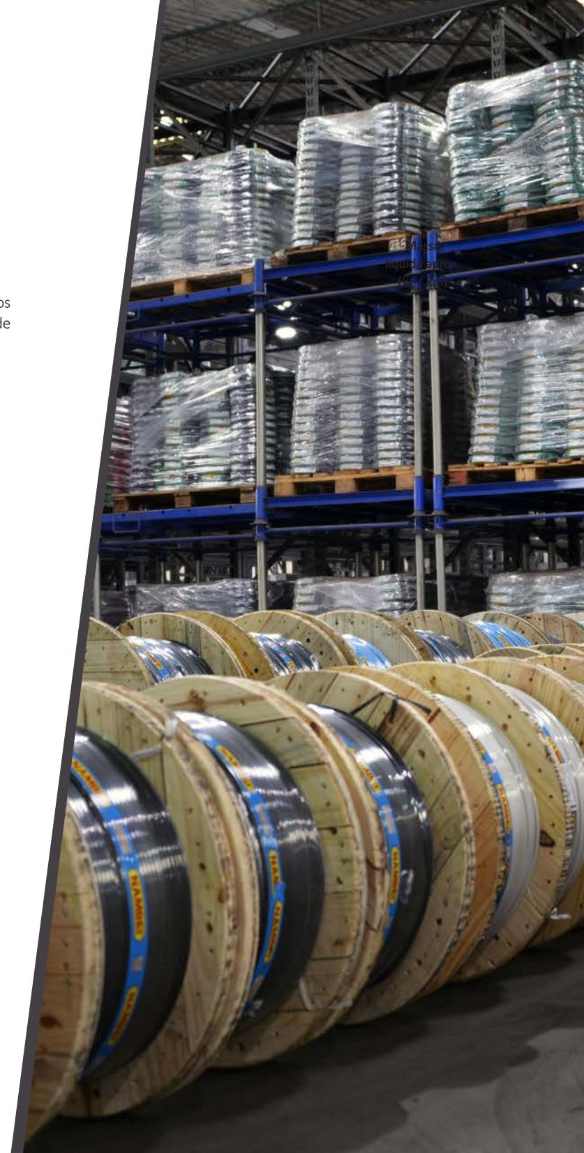
CABO NAMBEINAX FLEX HEPR ATOX 90°C MULTIPOLAR 0,6/1 kV
